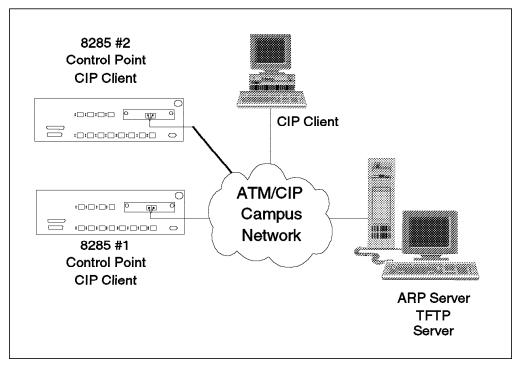
Figure 41. Multi-Switch CIP Network - Logical View
